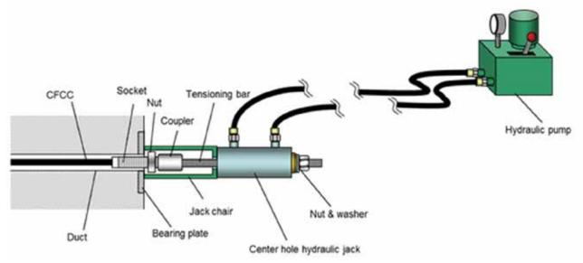
Fig. 3—Post-tensioning procedure.
