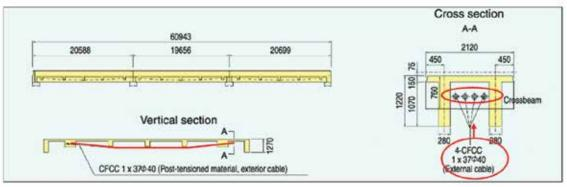
Fig. 6—Bridge Street Bridge cables. (Note: All dimensions in mm; 1 in. = 25.4 mm.)
