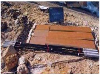
Exposure test and deterioration of sampled specimens at year 3Steel strFig. 15—Exposure test of newly developed ground anchor system using CFCC.
