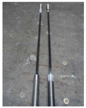
CFCC strands with pre-installed anchoring devices *Fig.* 17—*Research test configuration.*
